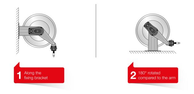
In the suitable open **series 530, 540 and 560** the rewinding brake can be installed as you like in the following three positions:
